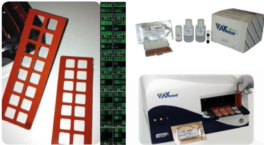
Figure 1| The VXI sHA assay is a new alternative potency assay to measure the concentration of functional hemagglutinin (HA). HA has been established to be the key component of whole virus vaccines and the dominant target of protective antibodies following vaccination or infection. Multiple influenza strains can be quantified within 2 hours. The VXI platform is comprised of the Influenza Seasonal Hemagglutinin Potency Assay Kit and the VaxArray Imaging System.
